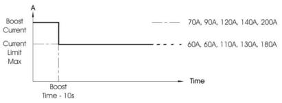
The drive boost current can be set in 1A steps between 10 and 140A but not less than the 'current limit max' setting, and the drive boost time to be altered in 1 second steps between 0 and 10 seconds.
