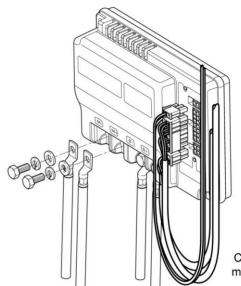
Cables should be mounted as shown
