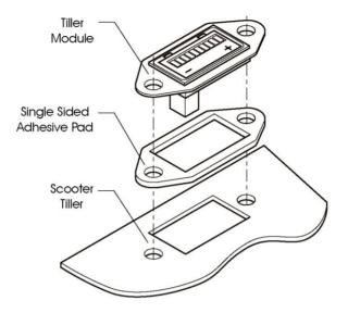
When correctly fitted this arrangement will give the Tiller Module an IPX5 ingress protection rating.
